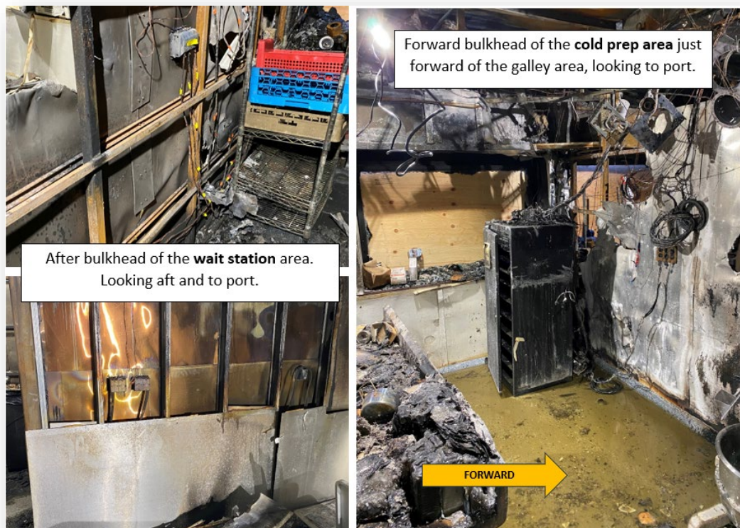
Figure 28 - Left , Images of the wait station area showing the structure and electrical circuits in the area identified as where the fire started. The yellow tape in the top left, are the result of forensic examination of the wiring conducted by investigators. Right , Image of the damage to the cold prep area just behind the wait station area. In both these images, material has been removed from the scene to facilitate examination of the scene. (Source: USCG)
