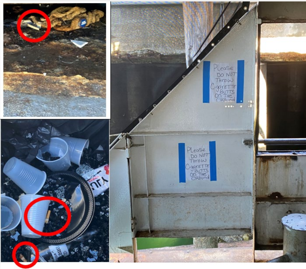
Figure 21 - Red circled objects are cigarettes located after the fire on the main deck and in rubbish from the vessel. Right , signage on the inside of the port main deck bulkheads indicating shipboard policy regarding cigarette butts. (Source: Coast Guard)
