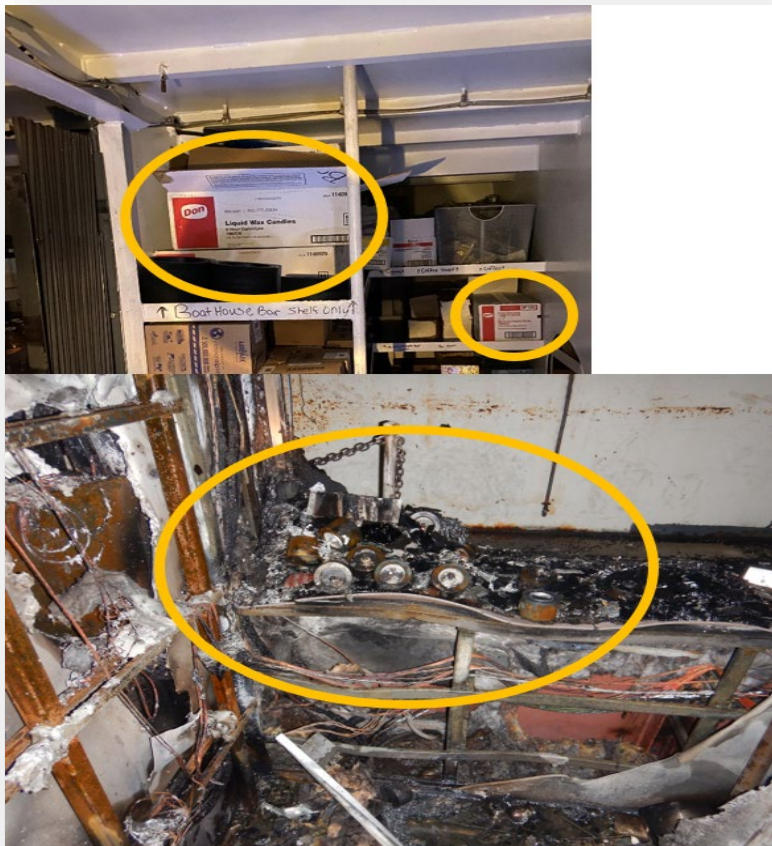
Figure 15 - Top: paraffin candles stored in racks near the galley area. Bottom: Fire-damaged canister fuel heating cans stored on the wide windowsill running fore and aft in the main deck wait station. (Source; USCG)
